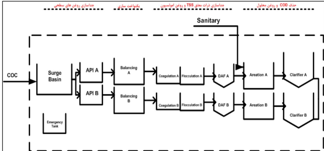
Figure 2: The stages of waste water treatment plant in Mobin Petrochemical Company
