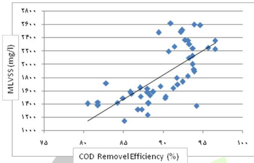
Figure 3: The relation between MLVSS and COD Removal Efficiency.
