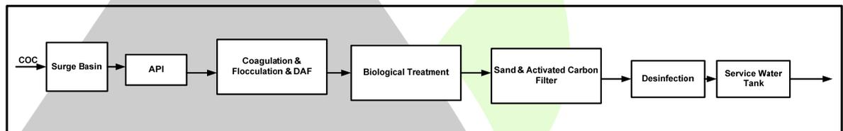
Figure 1: The sequence of waste water treatment plant in Mobin Petrochemical Company
