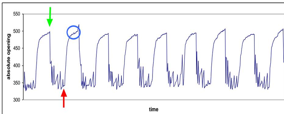
Figure 2. Movement behaviour (opening and closing of the valves) of fouling bivalves detected by a valve movement monitor during a P-C regime. Top arrow (green) indicates the start ('on'), the bottom arrow (red) the timing of stop ('off') of chlorination. The circle indicates the recovery period during which the bivalve slowly opens. Normal behaviour would reflect a continuously open valve position allowing respiration and feeding to occur.
