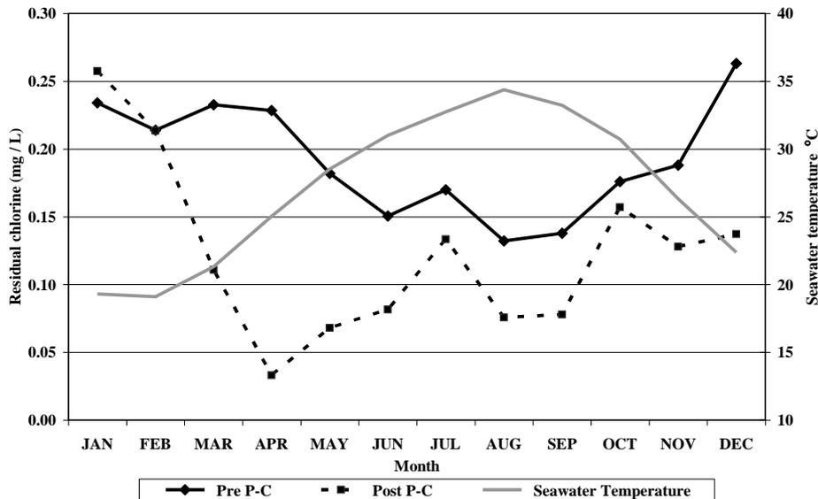
Figure 3. Monthly average data from on-line analysis of residual chlorine in the cooling seawater prior to release through back pressure weir into open channel leading to the sea. Data represents Pre P-C (2002-2007) versus post P-C (July 4th 2007 to 2008). Seawater temperature taken from seawater intake within RLP displayed.
